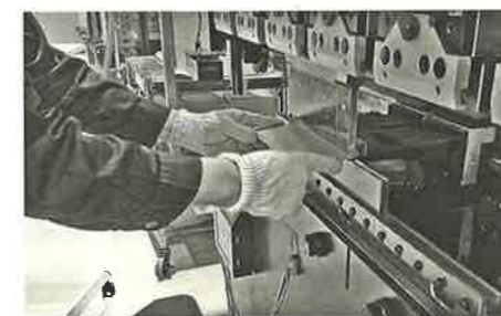
Fig.3 Mechanical sheet metal processing of test specimens
