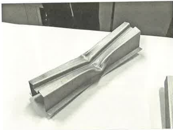
Fig.20 Deformation of test piece (design example 2)
