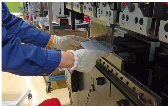
Fig. 3 Mechanical sheet metal processing of test specimens
